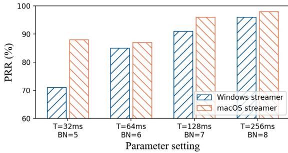
Fig. 10: Packet reception ratio with different streamer environments
