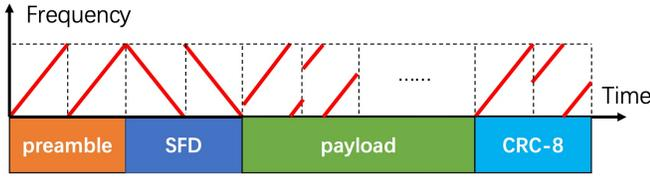
Fig. 4: The structure of the embedded packet
