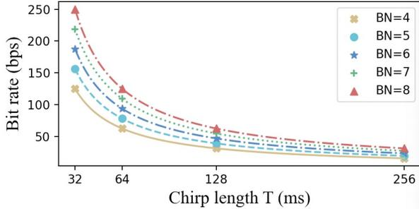
Fig. 9: Data rate under different  $BN$  and  $T$  settings
