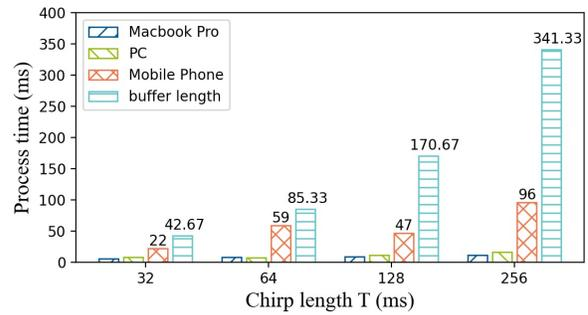
(a) Longest processing time for each buffer compared with buffer length
