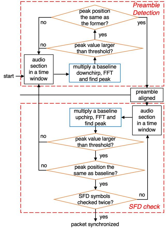
Fig. 5: Packet synchronization process
