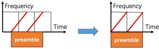
Fig. 6: Align chirps of the preamble with time window
