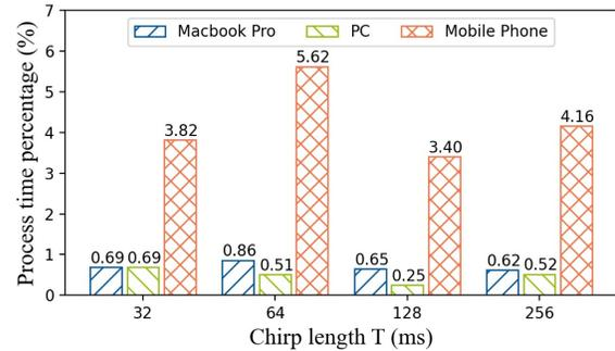
(b) Percentage between mean processing time for each buffer and the buffer length
