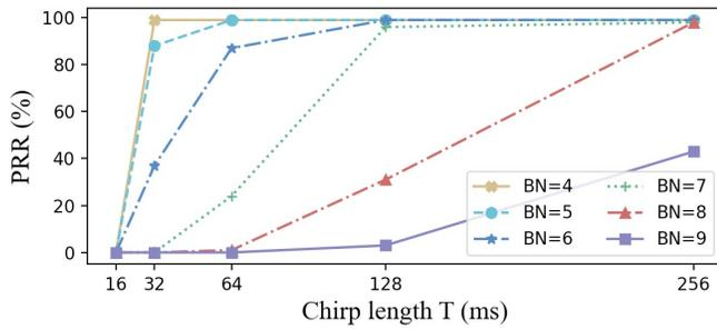
Fig. 8: Packet reception ratio under different  $BN$  and  $T$  settings
